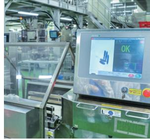
Equipment such as metal detectors and X-ray inspection apparatus keep out impurities.
